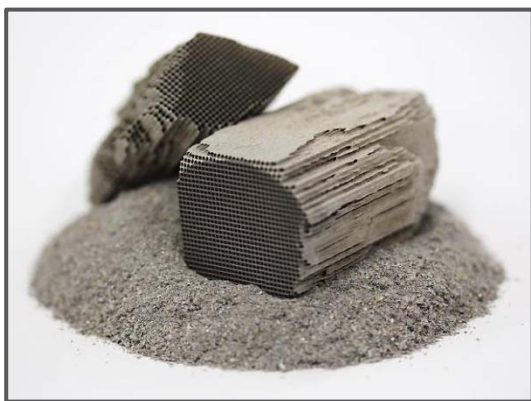
Figure 1: Platinum Group Metal Coating in Catalytic Converters for Automobile Emission Control
