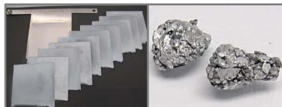
**Figure 2: High Purity Electrolytic Zinc Metal and Indium Sponge Produced from Pilot Program on Bulk Sulphide Concentrate**
